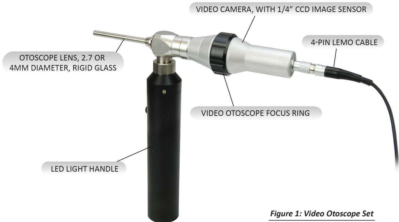
*Figure 1: Video Otoscope Set*
