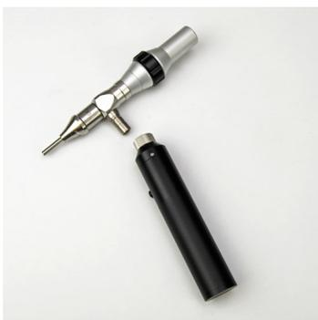
LED light handle in position to install on Otoscope.
