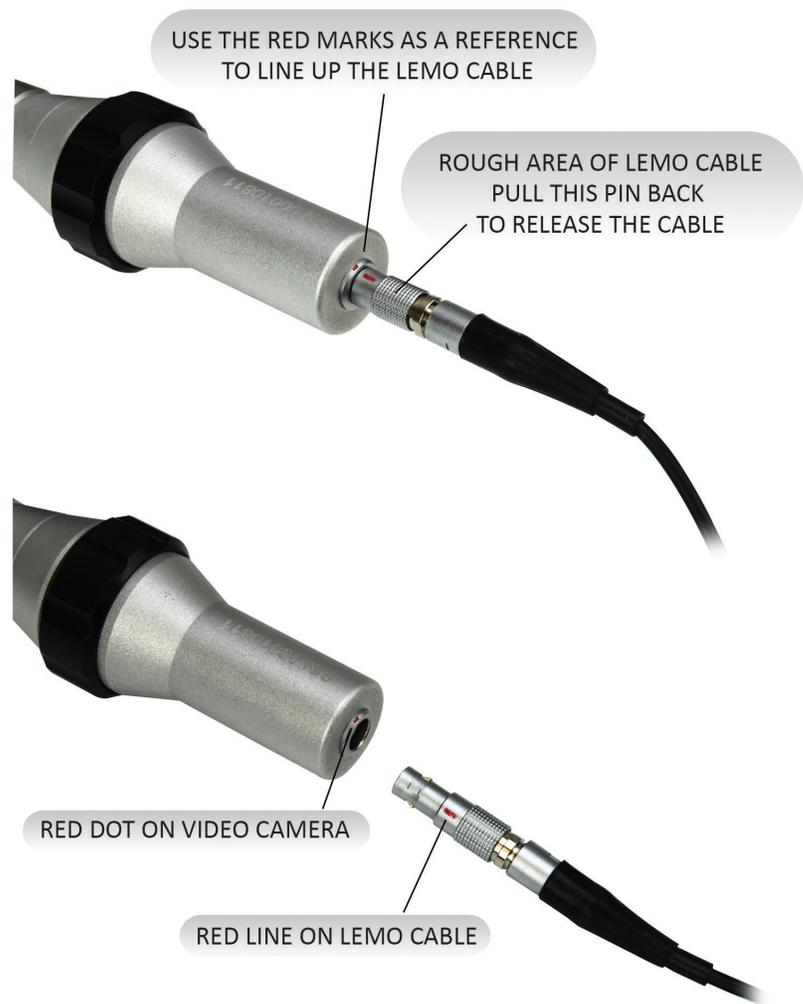
**Figure 2: Connecting & Disconnecting the Lemo Cable**
