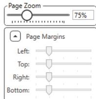
7. In the bottom left, the Page Margin is set by default to the ideal level. Adjusting this will determine how far items will print from the edges.
