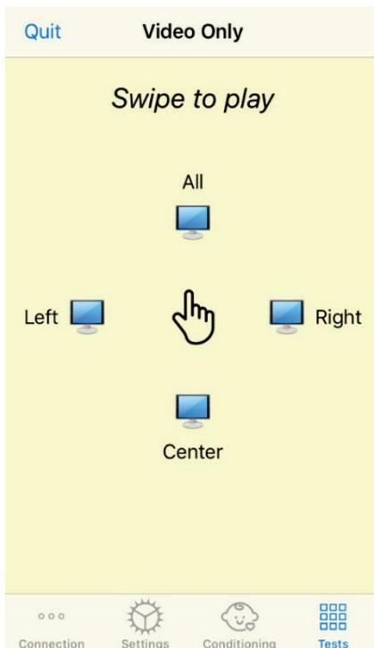
Video Only Mode, is designed for use with a separate audiometer. Video Only Mode will control the screens only. No stimulus is being presented and no thresholds are being recorded during this type of testing.
