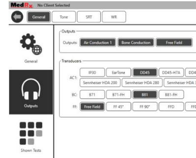
**Option 1:** On the General Options screen click Outputs to assign specific transducers to the audiometer outputs.
