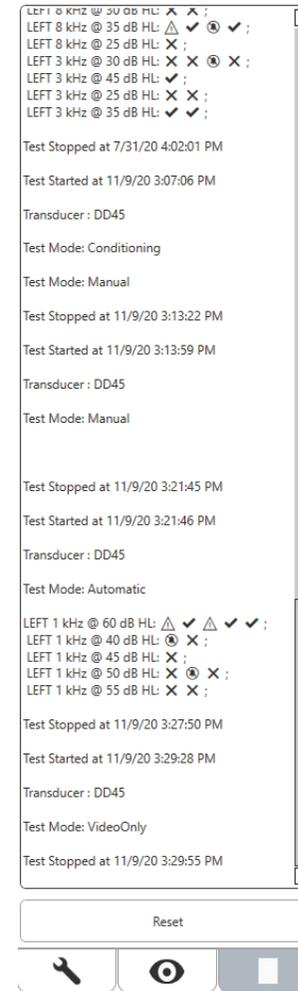
Testing information for both manual test mode and automatic test mode will be stored here. The following are what each log symbol means:
