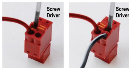
Place a small flat head screw driver on the small orange tabs and push down while inserting a speaker wire into the opening then remove the screw driver. Be sure the wire is secure.
