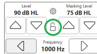
3. If you wish to maintain the balance of signal and masking (for example, masking always 30 dB above the signal), click the Lock button after setting the masking and signal levels.
