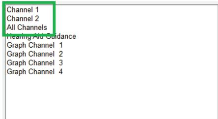
2. The “Channel” reports are the tinnitus assessment reports. Select the channel used for testing or All Channels when multi-channel testing is completed.
