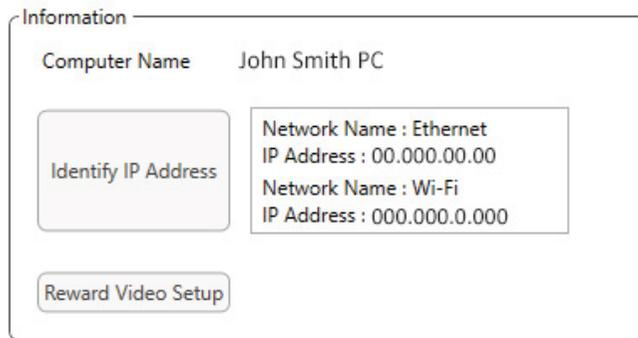
Studio will then list all available network connections. The VRA will need to be located on the same wireless network or Wi-Fi. On the iOS app, you can enter the computer name or Wi-Fi IP Address into the Server IP Address location
