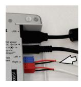
Notice! The Red & Blue adapters are included and must be removed to attach 18 gage (1.0mm) Free Field speaker wires and then reinstalled.
