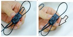
2. Install the hook on the back side of the probe mic. Pull hook down to seat on the post.
