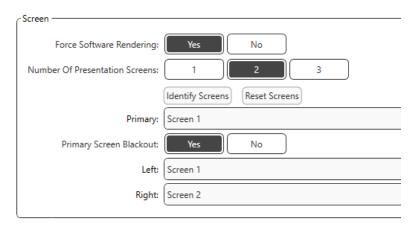
Click **Identify Screens** to determine which screen you would like as the left and right reward screen. These should be the screens that will be in the testing area where the child will be tested. If there are two monitors in the testing area the left and right monitors should be assigned in relation to the child's left and right ear.
