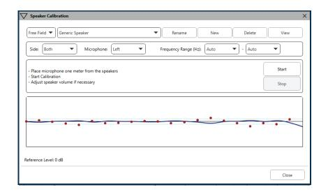
The speaker should be positioned in such a way that nothing blocks the path of the emanated sound in front and on the sides of the speaker. For example, positioning a speaker behind a monitor is incorrect and can severely affect its response at the measurement location. The speaker diaphragm should be at about the same level as the patient's ear and the reference microphone.
