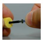
Place a new set of foam tips on the earphone tubes as shown. These tips are designed for single patient use and should not be washed and reused. NOTE: When removing foam tips after use, be sure the clear or black plastic tubing nipple remains attached to the long earphone tube.
