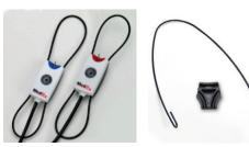
1. You will need the two Probe Mics, the Probe Mic Hanger and the clip.
