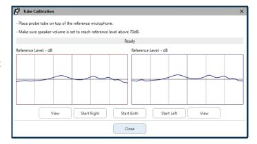
Position probe microphone between 19 and 39 inches from the loudspeaker and click Start Both to run simultaneously. The signal must be at least 70 dB to complete a valid calibration. If the screen prompt indicates the signal is too low, increase the volume on the loudspeaker or move the patient closer and restart the calibration.
