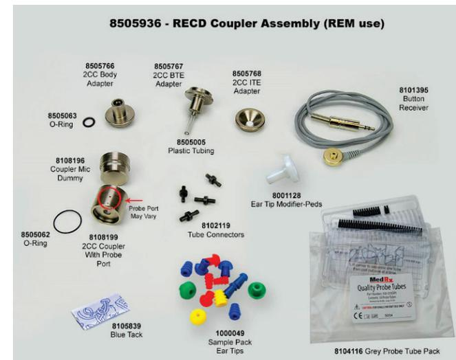
The RECD values are used as a correction to coupler measures for that client’s hearing instruments. By performing all subsequent measures in the coupler and applying the RECD corrections to the coupler measures, the “real ear” factors are incorporated into the results. The resulting simulated measurements provide information to select and make adjustments to the hearing instrument and verify adjustments in the MedRx coupler rather than
