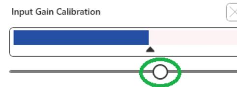
8. When using the Mic option adjust your input using the slider so that it is peaking at the black triangle under the VU meter.
