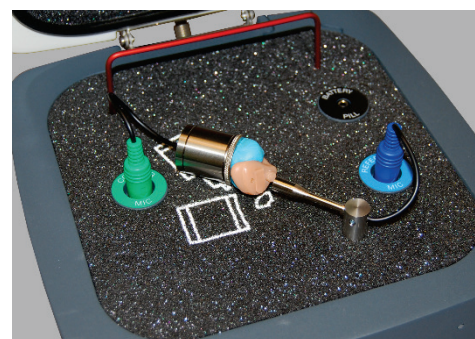
ITE Hearing Instrument
