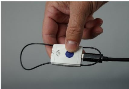
To prevent charging of the REM probes when not necessary in the MedRx Charger, inserting the probes into the device and then turning off the device.
