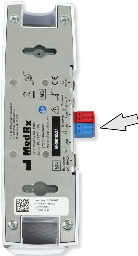
⚠ Notice! The Red & Blue adapters are included and must be removed to attach 18 gage (1.0mm) Free Field speaker wires and then reinstalled.
