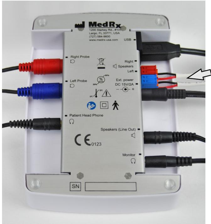
⚠ Notice! The Red & Blue adapters are included and must be removed to attach 18 gage (1.0mm) Free Field speaker wires and then reinstalled.
