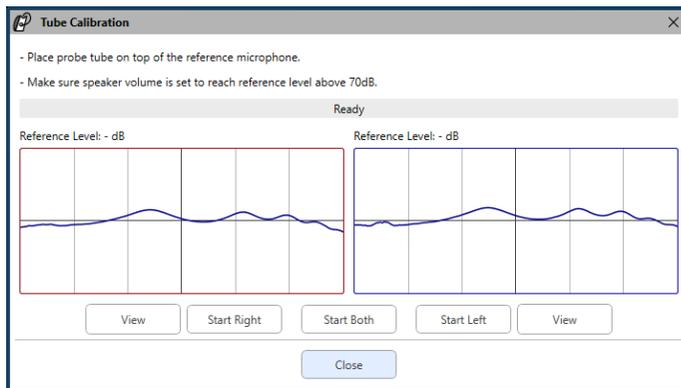
Position probe microphone between 19 and 39 inches from the loudspeaker and click Start Both to run simultaneously. The signal must be at least 70 dB to complete a valid calibration. If the screen prompt indicates the signal is too low, increase the volume on the loudspeaker or move the patient closer and restart the calibration.
