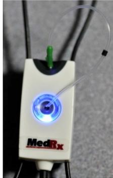
⚠ For reasons of infection control and reliability of results, MedRx recommends that a new probe tube be used with each patient. To ensure accurate measurements, it is necessary to calibrate the probe tube each time it is replaced.
