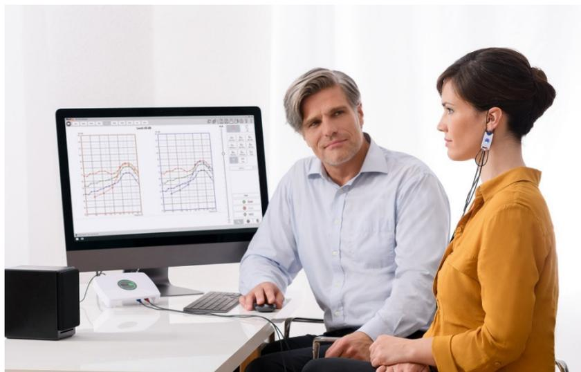
The AVANT REM+ and MedRx WREM are devices that are used in measuring the real ear acoustical characteristics of hearing instruments in-situ. The device performs measurements of real ear acoustical characteristics of a hearing instrument on a given human ear, and does comply with the International Standards ANSI S-3.46 and IEC 61669.
