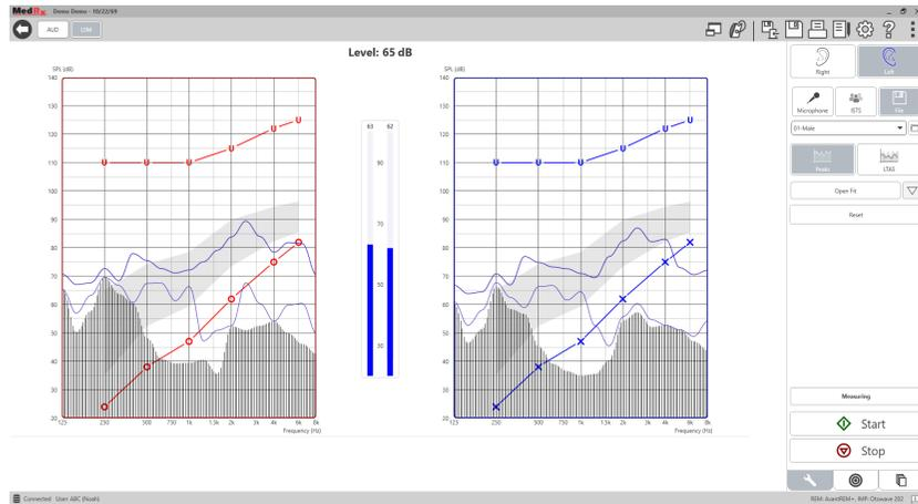
The Studio software provides several digital audio files to use as a repeatable stimulus for Speech Mapping. These are accessed by clicking the File button on the right and then selecting the desired track from the pull-down menu in the audio player. Peak measurements are recommended.
