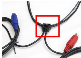
5. Turn clip over, place probe mic wires into clip.
