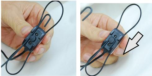
2. Install the hook on the back side of the probe mic. Pull hook down to seat on the post.
