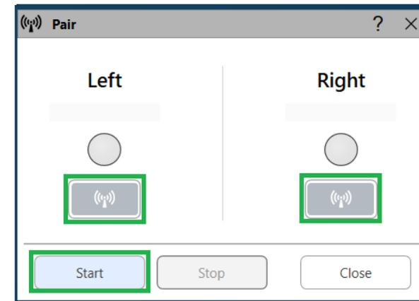
4. The Studio software will lightly fill the status circle (blue or red depending on earside) when a connection is established. The pairing is complete when the serial number is displayed in the pairing window. Confirm the serial number matches the probe you are trying to pair.
