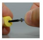
Place a new set of foam tips on the earphone tubes as shown. These tips are designed for single patient use and should not be washed and reused. NOTE: When removing foam tips after use, be sure the clear or black plastic tubing nipple remains attached to the long earphone tube.
