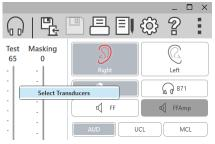
**Option 2:** You can change transducers by Right-Clicking on any transducer icon on the Audiometry screen.
