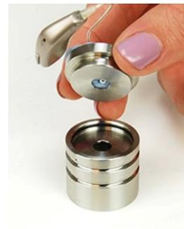
NOTE: If the RIC hearing aid has an earmold it can remain on the hearing aid and be attached to the coupler in the same method as an ITE hearing aid.
