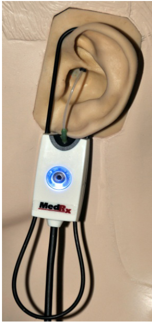
Probe Tube Insertion Guide for Live Speech Mapping and Conventional REM
