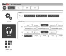
**Option 1:** On the General Options screen click Outputs to assign specific transducers to the audiometer outputs.
