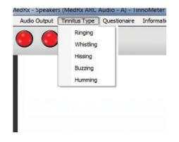
Start by selecting the tinnitus type that has been described by the patient. This is an approximation of the tinnitus sound your patient hears. Tinnitus type will provide a starting frequency, bandwidth and slope to help speed up testing time.
