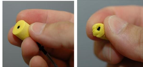
2. Carefully compress the tip between your fingers to allow it to fit into the patient's ear canal as shown. Do not roll the tip between your fingers.
