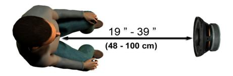
Proper positioning of the loudspeakers relative to the patient's hearing aids is critical for making accurate and repeatable measurements. Seat the patient so their ear is between 19 and 39 inches from the loudspeaker.
