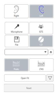
Select the CD button and then select a track. Use the sound level meter on screen to check the proper level. Adjust the output of the speaker to desired level using the sound level meter. (Remember conversational speech is 65 dB at 1 meter).
