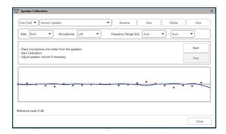
The speaker should be positioned in such a way that nothing blocks the path of the emanated sound in front and on the sides of the speaker. For example, positioning a speaker behind a monitor is incorrect and can severely affect its response at the measurement location. The speaker diaphragm should be at about the same level as the patient's ear and the reference microphone.
