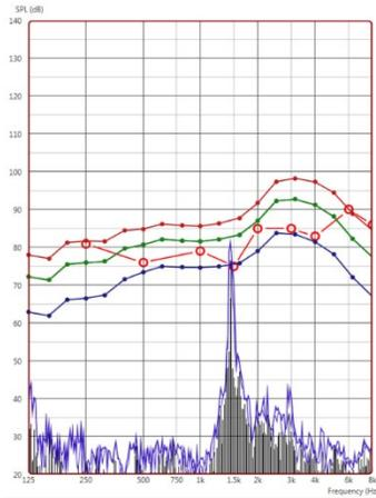
If a more specific frequency analysis of the feedback is desired, change the resolution of the system to 1/24 octave and adjust the smoothing in the General LSM or REM settings menu. This image shows the similar feedback as above at 1/24 octave, smoothing 1.
