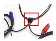
5. Turn clip over, place probe mic wires into clip.
