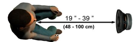
Proper positioning of the loudspeakers relative to the patient's hearing aids is critical for making accurate and repeatable measurements. Seat the patient so their ear is between 19 and 39 inches from the loudspeaker.
