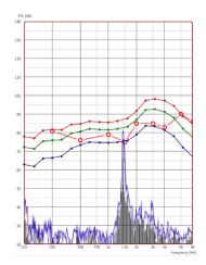
If a more specific frequency analysis of the feedback is desired, change the resolution of the system to 1/24 octave and adjust the smoothing in the General LSM or REM settings menu. This image shows the similar feedback as above at 1/24 octave, smoothing 1.
