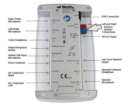
Notice! The Red & Blue adapters are included and must be removed to attach 18 gage (1.0mm) Free Field speaker wires and then reinstalled.
