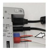
Notice! The Red & Blue adapters are included and must be removed to attach 18 gage (1.0mm) Free Field speaker wires and then reinstalled.
