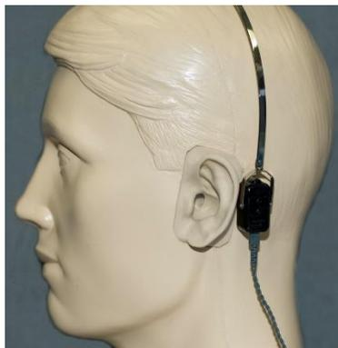
2. Establish bone conduction thresholds as described above (see page **Error! Bookmark not defined.**, steps 5-8) for 1000 Hz, 2000 Hz, 4000 Hz, 500 Hz and 250 Hz.
