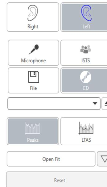
Select the CD button and then select a track. Use the sound level meter on screen to check the proper level. Adjust the output of the speaker to desired level using the sound level meter. (Remember conversational speech is 65 dB at 1 meter).
