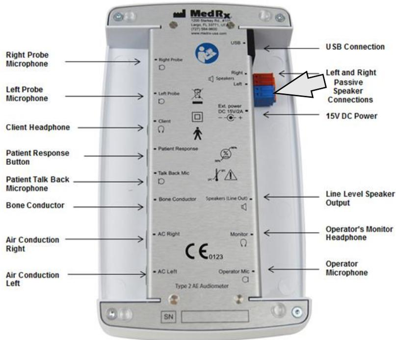
⚠ Notice! The Red & Blue adapters are included and must be removed to attach 18 gage (1.0mm) Free Field speaker wires and then reinstalled.
