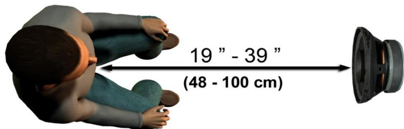
Proper positioning of the loudspeakers relative to the patient's hearing aids is critical for making accurate and repeatable measurements. Seat the patient so their ear is between 19 and 39 inches from the loudspeaker.
