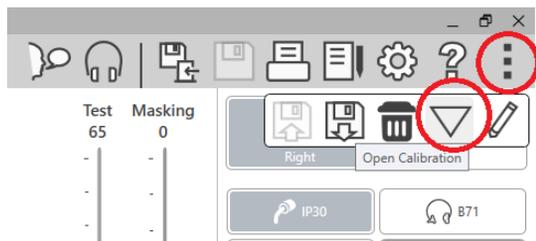
1. With the MedRx USB Flash Drive connected, open the MedRx Studio software, enter the module you will be loading calibration files into and click:
