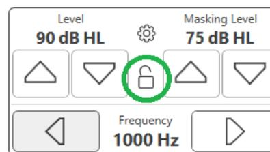
3. If you wish to maintain the balance of signal and masking (for example, masking always 30 dB above the signal), click the Lock button after setting the masking and signal levels.
