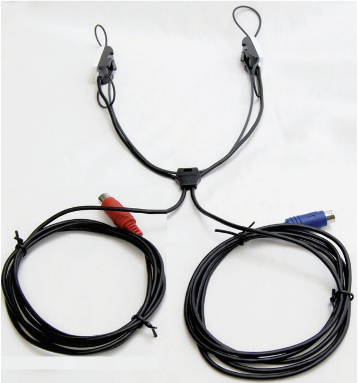
Probe Mic Hanger installation assembly complete.
