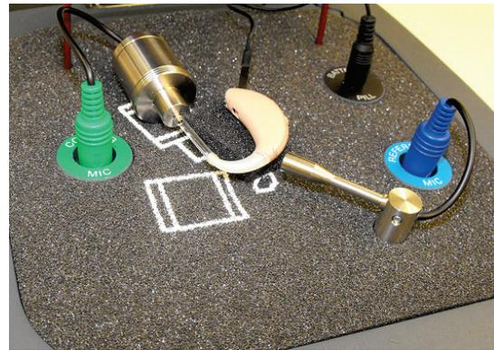
Place the aid on a foam pad or other material if needed to raise the sound inlet to the level of the reference microphone, with a 2 – 8mm separation distance.
