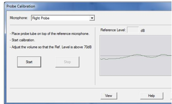
The calibration date is available under the **Function > Calibrate > Calibration Information** tabs. Return Probe Microphones to MedRx for annual re-calibration. Annual re-calibration ▼ of the Avant REM+ Probe Microphones is recommended. There are no user repairable components of this device.
