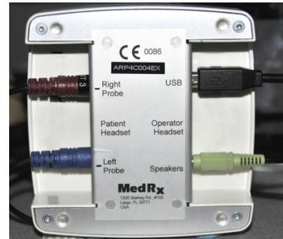
2. Connect the probe microphones to the AVANT REM Speech+ main unit as shown above. DO NOT force the connector into the jacks. Align correctly before insertion. A cable from the "Speaker" jack on the REM Speech+ will connect to the input jack in the powered speaker supplied with your unit.
