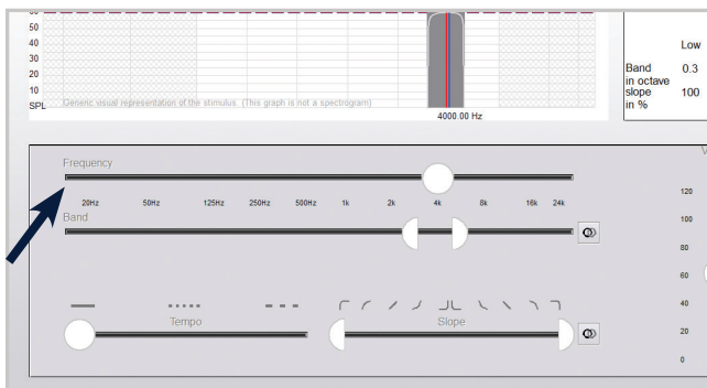
3. Match frequency level and band slope of tinnitus. Tempo will pulse sound to help with differentiation.
