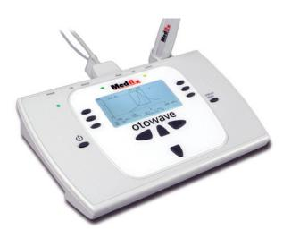
The 302+ offers six configurable patient profiles for faster middle ear measurements.
