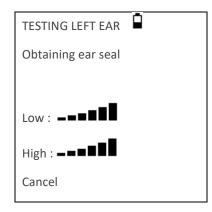
The number of bars shown indicates the robustness of the seal. The probe should be adjusted in the ear until two or more bars are shown for Low & High.
