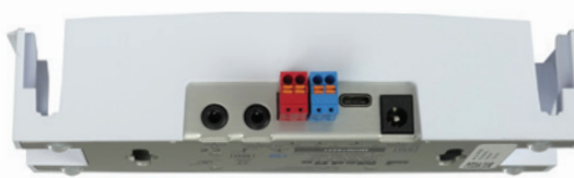
Backside of WREM Ports for: Monitor, Speaker (Line Out), Speakers - Right & Left, USB-C and Power
