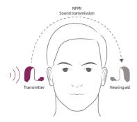
A transmitter with a microphone that wirelessly picks up and sends the sound from your poorer ear to the better ear.
