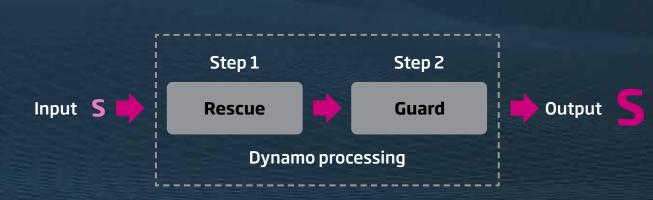
Step 1 "Rescue": In the signal path of the hearing instrument, high frequency components of the incoming sounds are first moved to lower frequencies through Speech Rescue.
