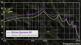
Full-On Gain measurements performed in technical settings according to ANSI S3.22-2003 (2cc coupler). Oticon Dynamo SP (purple) and other manufacturer (green). Both super power devices use size 13 battery.
