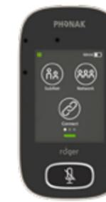
**Phonak Roger:** The Roger uses adaptive frequency hopping where transmission remains on a given frequency for a short time, and if interference is detected, the data will be re-sent later, when it "hops" to a different frequency.
