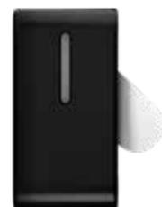
**The Oticon ConnectClip** was designed as a multi-function device that transmits to Oticon 2.4 GHz compatible hearing aids, allowing for hands-free calls, volume control of the hearing aids, and a remote microphone mode.
