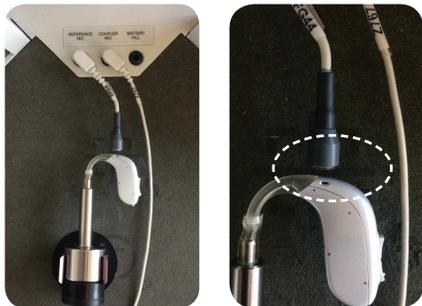
Figure 9: Position of hearing aid and microphone in Verifit-1
