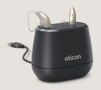
The all-new desktop charger for Oticon Intent has been redesigned to be smaller and lighter, with more visible left and right markings. It provides fast charging that is done through contact charging for improved reliability.
