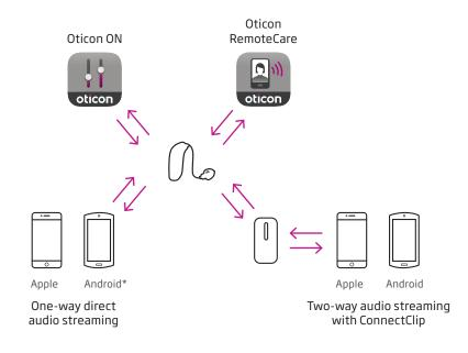
\* One-way direct streaming from Android is only possible with Oticon More hearing aids and if the mobile device supports ASHA.
