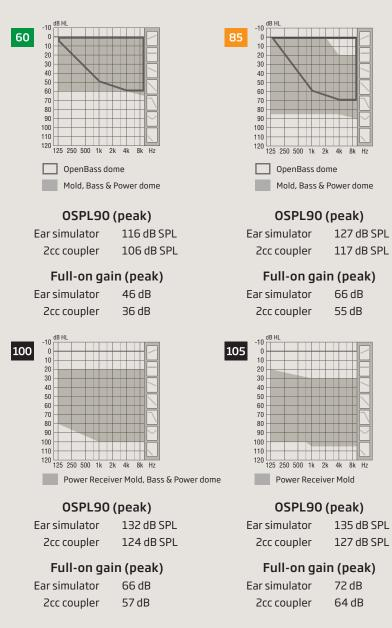
\* Fitting range is based on Oticon More 1. Fitting range for Oticon More 2 & Oticon More 3 is limited to 8 kHz. Details available in Technical data sheets.
