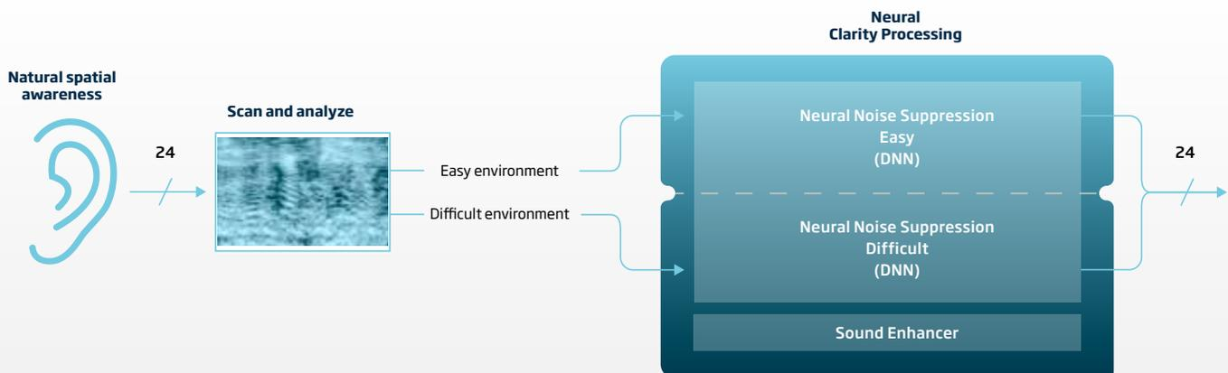
Figure 1: The processing flow of MoreSound Intelligence in single-microphone hearing aids.
