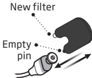
Insert the empty pin into the wax filter in the speaker and pull it out.
