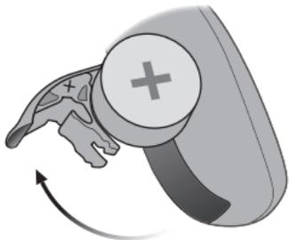
Fully open the battery drawer and remove the battery.
