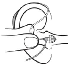
Hold the bend of the speaker wire between your thumb and index finger.
