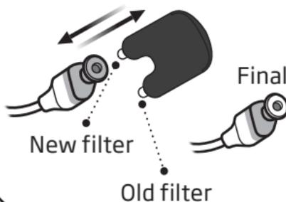
Insert the new wax filter using the other pin. Remove the tool and throw it out.
