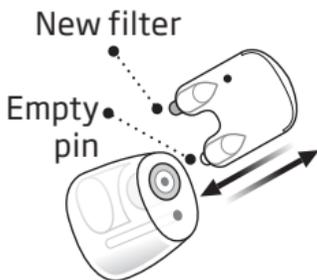
Insert the empty pin into the wax filter in the earpiece and pull it out.
