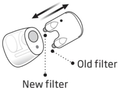
Insert the new wax filter into the wax filter in the earpiece using the other pin. Remove the tool, and throw it out.
