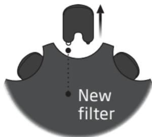
Remove the tool from the shell. The tool has two pins: one empty for removal and one with the new wax filter.
