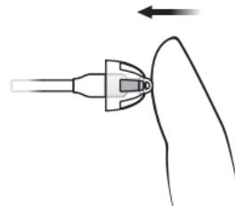
Push firmly to ensure that the earpiece is securely fastened.
