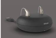
miniRITE R offers a discreet design powered by a rechargeable lithium-ion battery. The inductive charger secures reliable and fast charging within 3 hours for a full charge.
