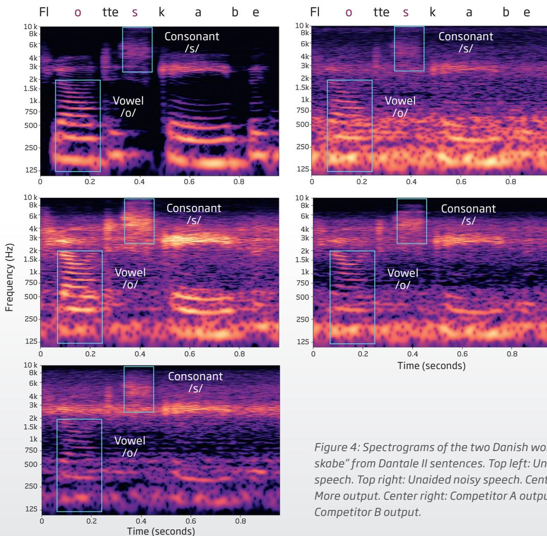
Figure 4: Spectrograms of the two Danish words "flotte skabe" from Dantale II sentences. Top left: Unaided clean speech. Top right: Unaided noisy speech. Center left: Oticon More output. Center right: Competitor A output. Bottom left: Competitor B output.
