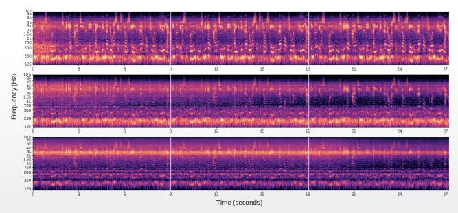
Figure 5: Spectrograms generated from the first 27 seconds of output recordings of Oticon More (top), Competitor A (middle) and Competitor B (bottom).
