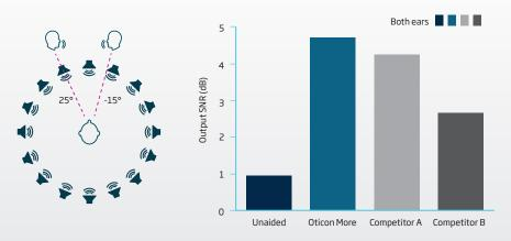
Figure 2: Schematic illustration of talker positions and SII-weighted output SNRs in dB measured in the lunchroom scene.
