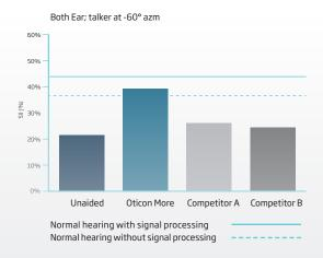
Figure 7: The calculated Speech Intelligibility Index (SII) from the Cafe scene of the different devices (and unaided) for an N3 audiogram (bars) and for normal hearing thresholds (lines).
