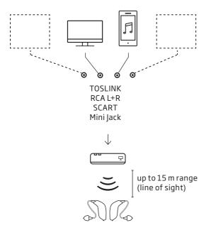
The TV Adapter 3.0 wirelessly transmits real-time stereo audio from a TV, home entertainment system or other audio devices directly to Oticon hearing aids at a distance of up to 15 meters. The child can set the volume to their preferred level for a listening experience free from the distraction of surrounding noise. In Oticon ON App the volume of the sound streamed from the TV can easily be adjusted.
