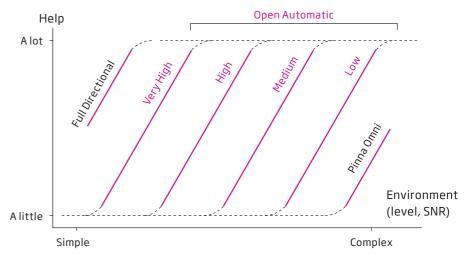
Open Sound Transitions. Open Automatics adapts to the acoustical conditions based on one of the four transition profiles: Very High, High, Medium, or Low. Pinna Omni does not balance speech and noise sources but gives equal focus to all sounds even in complex listening environments. Full Directional focuses on sounds coming from the front.
