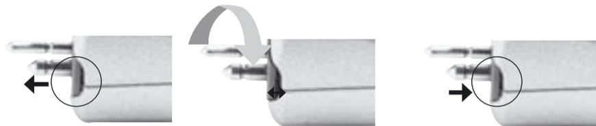
Note: Never use force when changing the pin orientation, as the pins will be permanently damaged if over-rotated.
