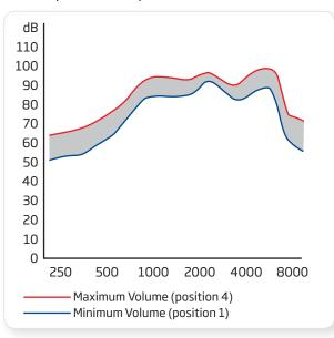
\*Measured with Corda<sup>2</sup> tube size 1.09 attached to 2 cc BTE Coupler, Amigo T30 transmitter and lapel microphone
