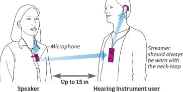
The Microphone will transmit the speech from the Speaker directly to the Hearing instrument user.
