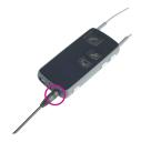
Connect the mini jack end of the interface cable to the Streamer Pro's mini jack. On the top of Streamer Pro, the on/off indicator should be green (indicating Streamer Pro is on), and the status indicator should be orange (if not, press the AUX button).
