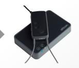
Place the Streamer Pro next to or on top of the Phone Adapter 2.0. The pairing will take approximately 20-60 seconds. The light will turn steady blue when the pairing is completed.
