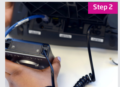
Remove phone receiver cord from phone base & replace with coiled cable from Sennheiser box. The coiled phone cable will now connect the Sennheiser box and phone base.
