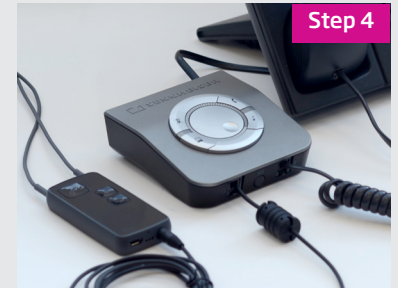
Insert the AUX cable into the headset jack on the Sennheiser device as pictured. Plug the mini jack end into Streamer Pro.*
