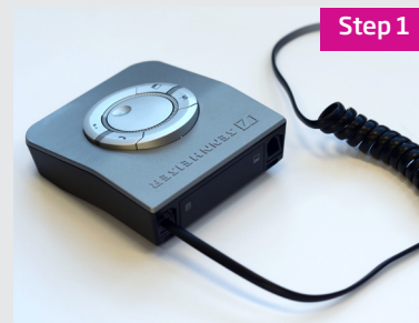
Insert coiled cable into the back port of the Sennheiser box as pictured.
