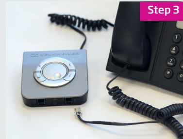
Insert phone receiver cord into front of Sennheiser box.
