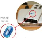
**STEP 1:** Place Streamer close to adaptor. Press pairing button until blue light flashes rapidly.
