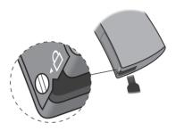
Use the screwdriver to turn the screw to unlock position (vertical). Insert the screwdriver into the slit in the bottom of the hearing instrument and push the door open.
