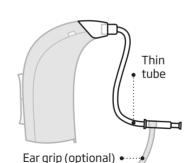
thin tube will have one of the following ear pieces - dome, GripTip, micro mold, or LiteTip.
