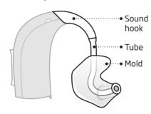
BTE with thin tube (Corda miniFit) An instrument with a
