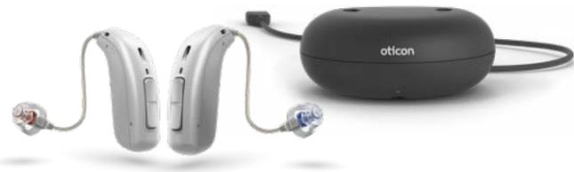
Oticon Opn Play miniRITE R is a discreet rechargeable style with a lithium-ion battery and easy-to-use charger. The wireless charging is based on inductive technology and enables reliable and fast charging in just 3 hours for a full day of hearing, including streaming\*. A quick recharge of 30 minutes gives an additional six hours of power. If a replacement is needed, the lithium-ion battery is easy to replace in the clinic. No need to send in for service.
