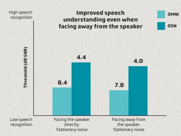
A speech recognition test in noise was used to see whether children would receive comparable benefit with OpenSound Navigator when the listener faced the speaker directly as well as away from the speaker.
