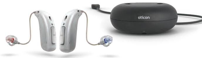
Oticon Opn S miniRITE R is a discreet rechargeable style with a lithium-ion battery and easy-to-use charger. The wireless charging is based on inductive technology and enables reliable and fast charging in just 3 hours for a full day of hearing, including streaming.\* A quick recharge of 30 minutes gives an additional six hours of power. If a replacement is needed, the lithium-ion battery is easy to replace in the clinic. No need to send in for service.
