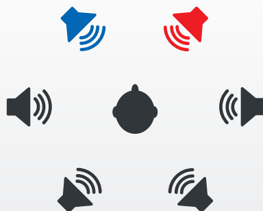
Figure 3. Test setup with a total of six loudspeakers. There are two target speakers in the front (in blue and red, at +/- 22 degrees). Each of the remaining four loudspeakers (in black, at +/- 90 degrees and +/- 150 degrees) presents a 4-talker babble, resulting in a 16-talker babble. All loudspeakers are placed 141 cm from the participant.
