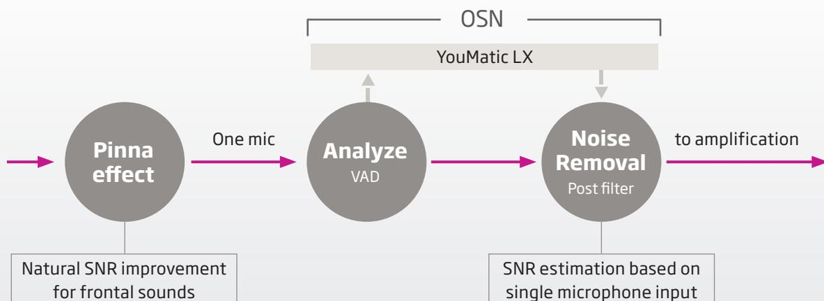
Figure 1: Modules in the single microphone OpenSound Navigator.
