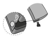
Use the screwdriver to turn the screw to unlock position (vertical). Insert the screwdriver into the slit in the bottom of the hearing instrument and push the drawer open.
