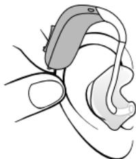
Gently pull your ear outwards and press the mould in the direction of the ear canal, twisting it slightly.
