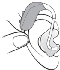
Gently pull your ear outwards and press the earmold in the direction of the ear canal, twisting it slightly.
